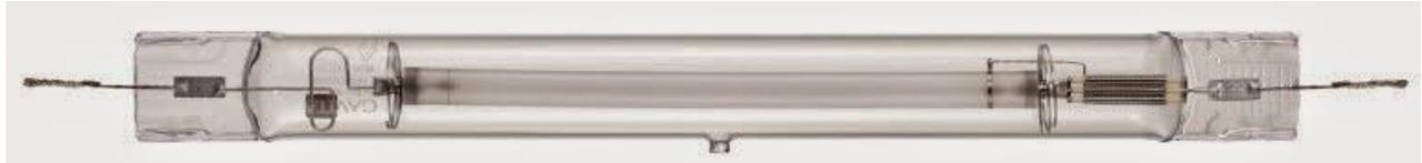
This is a double ended lamp. It doesn't have a threaded base that screws into a normal mogul socket. It has two braided wires coming off either side of it. These lamps are made of quartz so you **NEED TO WEAR GLOVES WHEN HANDLING**. Unlike normal High Pressure Sodium and Metal Halide bulbs, you cannot touch the glass on these bulbs with bare hands. If you get moisture or oil from your fingers on quartz glass, when the bulb heats up it can heat up the oil and cause the bulb to break.
