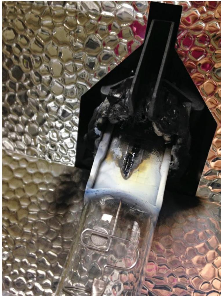
This is what can happen if your lamp is improperly installed. In this case, the wires did not make full contact with the metal and the socket was not slid 100% forward to hold the bulb in place. The electrical current arced, burnt up the lamp and melted the socket. This is the best-case scenario, it could have been much worse.
